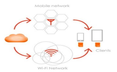
By offloading users from the 3G/4G network to Wi-Fi networks, mobile operators can add more capacity in an affordable and flexible way. Both subscribers and devices tend to connect to Wi-Fi whenever it is in reach.
