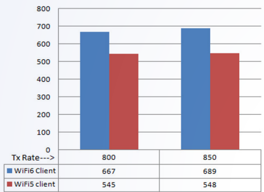
DL UDP Throughput Comparison between WiFi 6 & WiFi 5 single client in TS1
